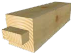
Tenon (with mitered shoulders)
