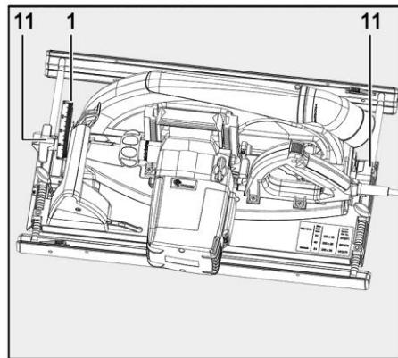
Fig. 17: Setting the saw unit for bevel cuts
