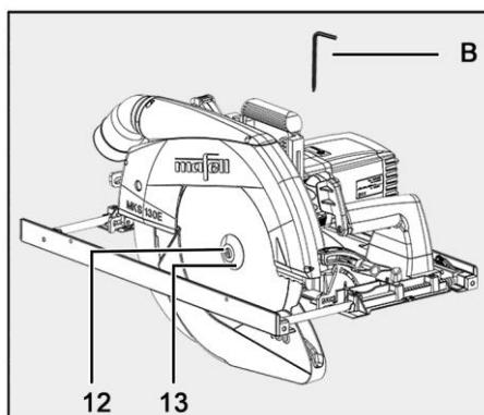
Fig. 8: Removing flange screw and clamping flange
