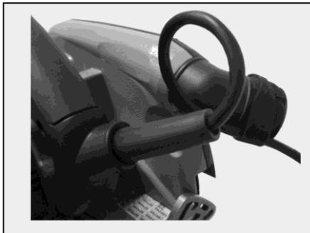
Fig. 6: Routing the connecting cable
