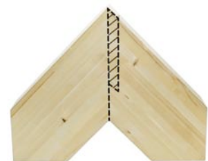
Possible type of assembly (rafter to rafter without ridge purlin)
