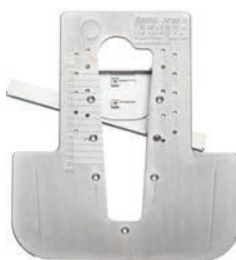
Fence fitted on the female plate
