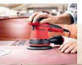
For fine sanding and when sanding between coats, a stroke of 3 mm makes the EVA 150 E/3 particularly adept.
