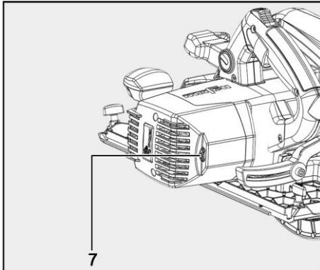
Fig. 15: Selecting the rotational speed at the setting wheel
