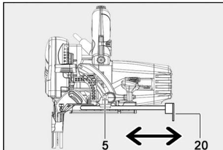
*Fig. 24: Adjusting the cutting width via the parallel guide fence*
