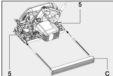
*Fig. 23: Installing the parallel guide fence***Use the following procedure to adjust the cutting width:**
