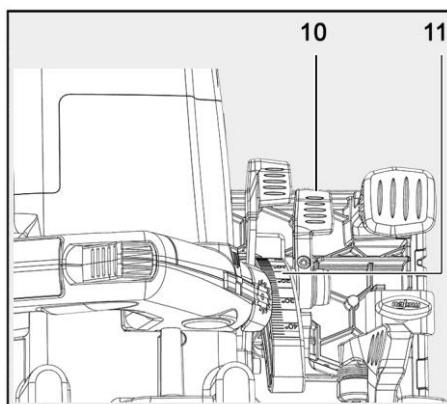
Fig. 18: Setting the saw unit for bevel cuts
