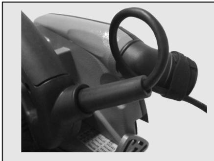
Fig. 6: Routing the connecting cable
