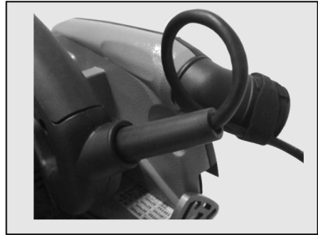
Fig. 6: Routing the connecting cable
