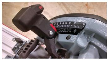
5 Squeeze-operated depth-setting lever and scales off and on track.
