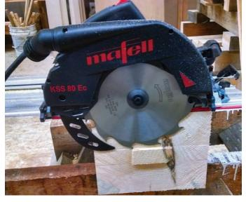
3 In-track depth of cut is 3½ in. Riving knife descends with blade to keep kerf open behind blade. Dust chute rotates and accepts hose.
