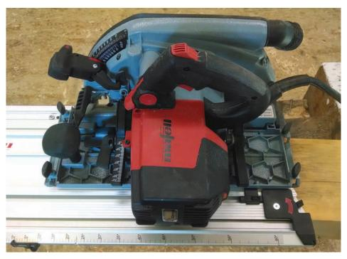
1 Saw releases from track via single lever, lower right. Auto-return fitting just forward. Depthsetting lever at upper left frees by squeezing button, locks at new position upon release. Blade guard retractor just beneath. Fence-rod housings with twin thumbscrews at ends of cast base.
