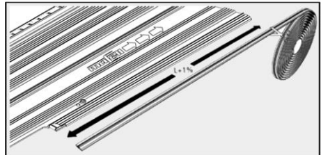
Fig. 12: Inserting the new chip breaker guard
